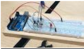
Figure 16 - Blinking LED from a different angle. This picture represents the final result of the Blinking LED Circuit
